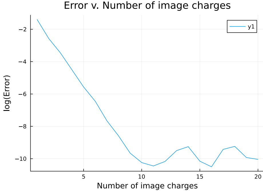
Figure 3.2: The error as we add more image charges, with the image charges being distributed on a circle of radius .1 around (0,-1)
