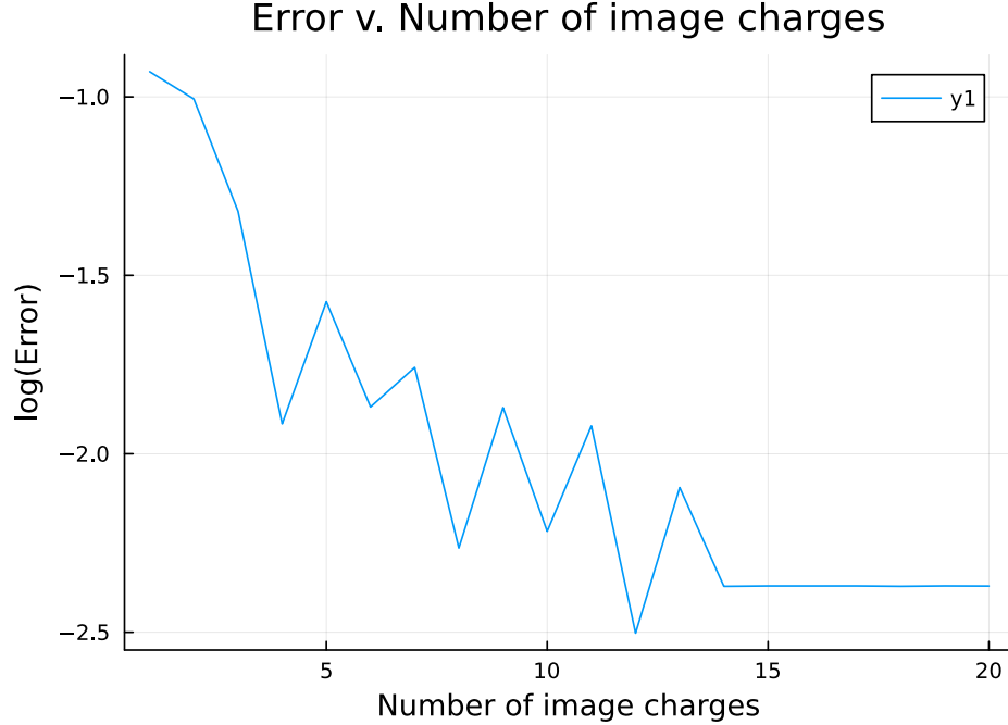
Figure 3.4: The error as we add more image charges, with the image charges being distributed on a circle of radius .1 around (0,-0.7)
