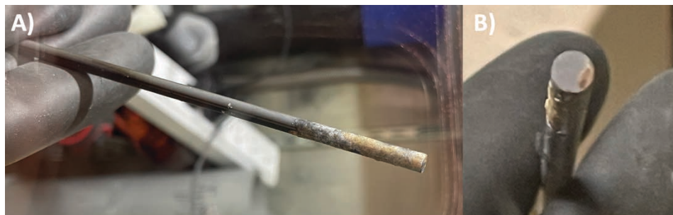
Figure 6.18 UCl 3 in LiCl-KCl at 450 °C.
