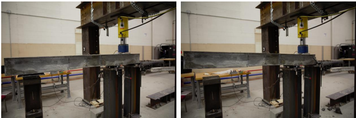
Figure 6.15 M468R tie at start and end of loading
