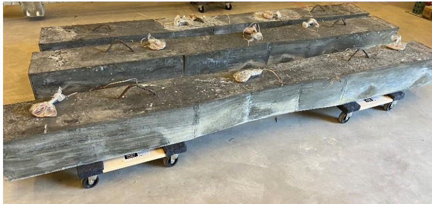
Figure 6.7 UHPC tie specimens after removed from formwork
