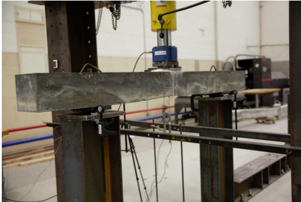
Figure 6.9 Actual test setup for railway tie specimen under negative center point bending
