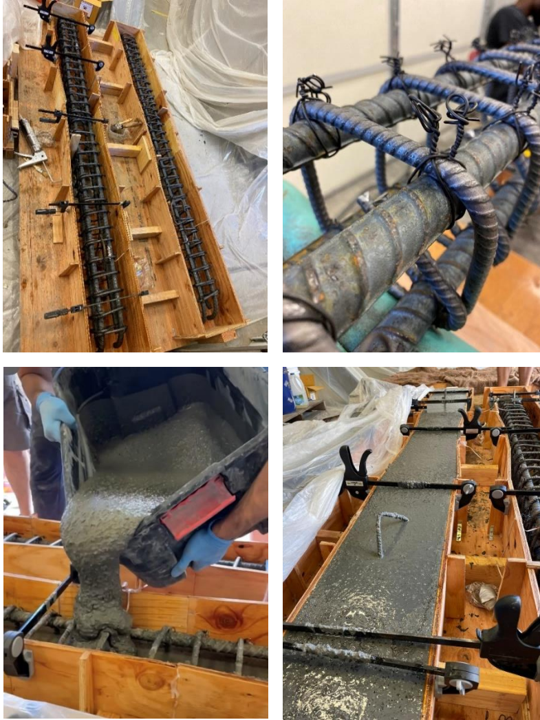
Figure 6.5 Fabrication of UHPC tie specimen
