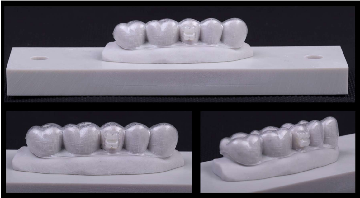
Figure 2.15: Testing aligner positioned on final testing model
