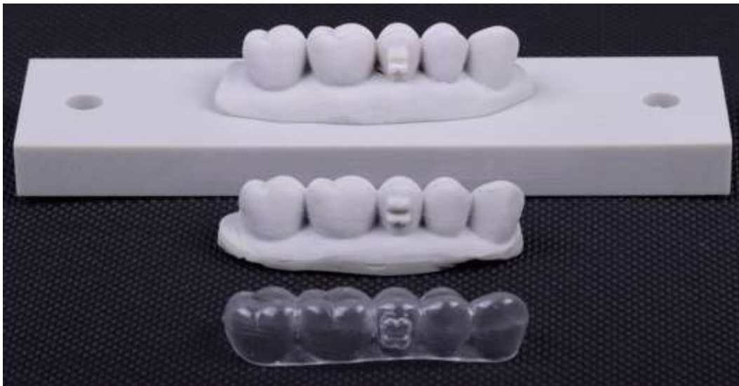
Figure 2.14: Final testing model with UL5 bracket bonded
