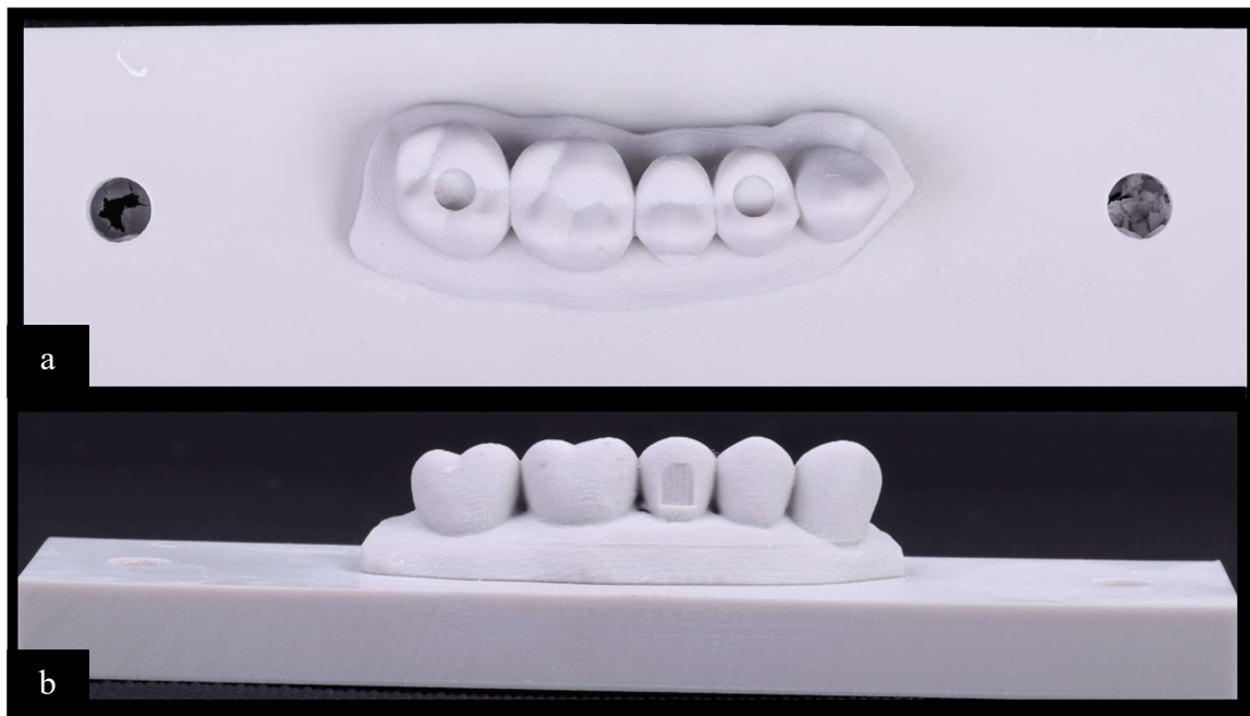
Figure 2.11: 3D printed testing model prior to bracket placement a) occlusal view b) side view
