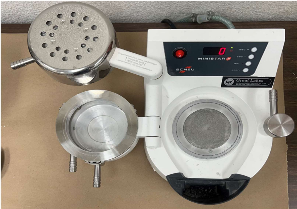
Figure 2.4: MiniStar S pressure forming machine used during entire investigation for fabrication of vacuum-formed aligners
