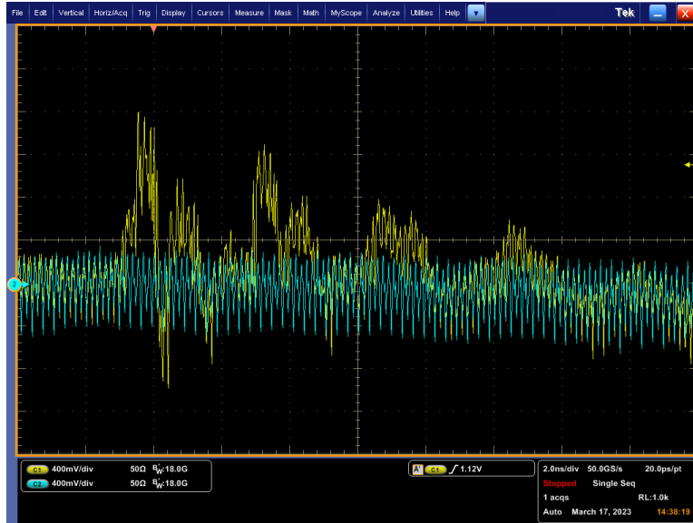
Fig. D.46 An oscilloscope capture is taken from the experimental setup demonstrated in Fig. D.44 where the linear antenna waveguide structure is placed external to an AWG 4 on a fixed axis translated at z = -17.8\text{cm} .
