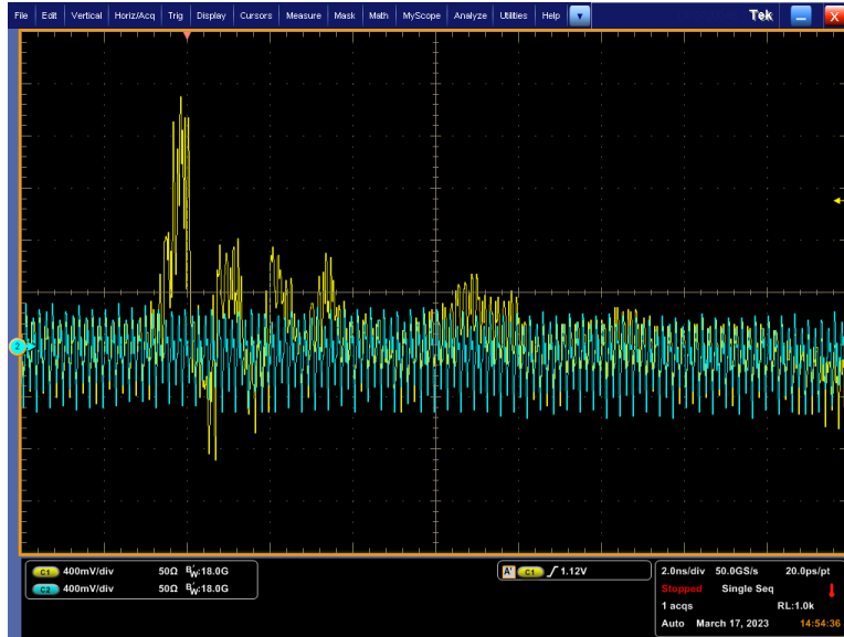
Fig. D.48 An oscilloscope capture is taken from the experimental setup demonstrated in Fig. D.44 where the linear antenna waveguide structure is placed external to an AWG 4 on a fixed axis translated at z = -2.5\text{cm} .
