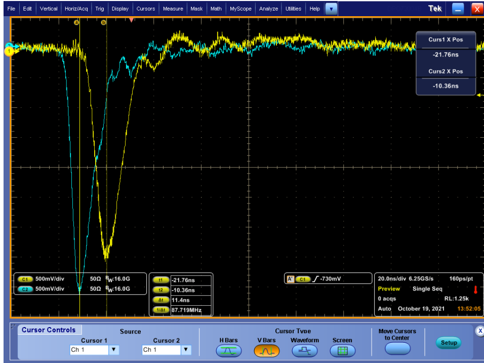
Fig. 3.41 The “output monitor” of the Bournlea Instruments Pulse Generator is indicated by channel 1 (yellow) of the oscilloscope. The HV output is indicated by channel 2 (turquoise) of the oscilloscope. The “output monitor” of the pulse generator is internally attenuated by 60dB and additionally attenuated with a 20dB attenuator ( 80dB total attenuation). The HV output is forced to be attenuated by 80dB using attenuators. There exists a difference in time delay of about 10ns between peaks despite having the same length of cable connections. There is also an amplitude difference between pulses of about 500mV (or 500V non-attenuated) despite having 50\Omega terminations on the oscilloscope. For experimental purposes, the HV output is fed into the mock DPF, and the “output monitor” is used as a trigger for the oscilloscope.
