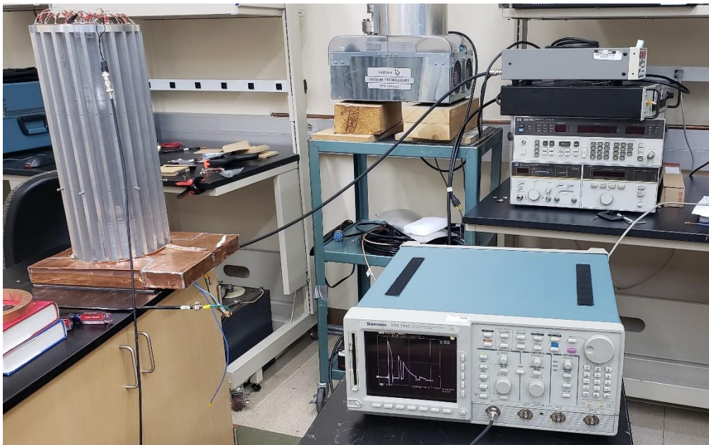
Fig. 4.5 From Section 3.3.1, an experiment was performed to fire a 12V , 121\mu s pulse into the base of the mock DPF. An oscilloscope is connected across the pinch end of the mock DPF with high impedance to measure the pulse signal. This experimental result can be compared to the simulation data seen at the pinch end of the mock DPF.
