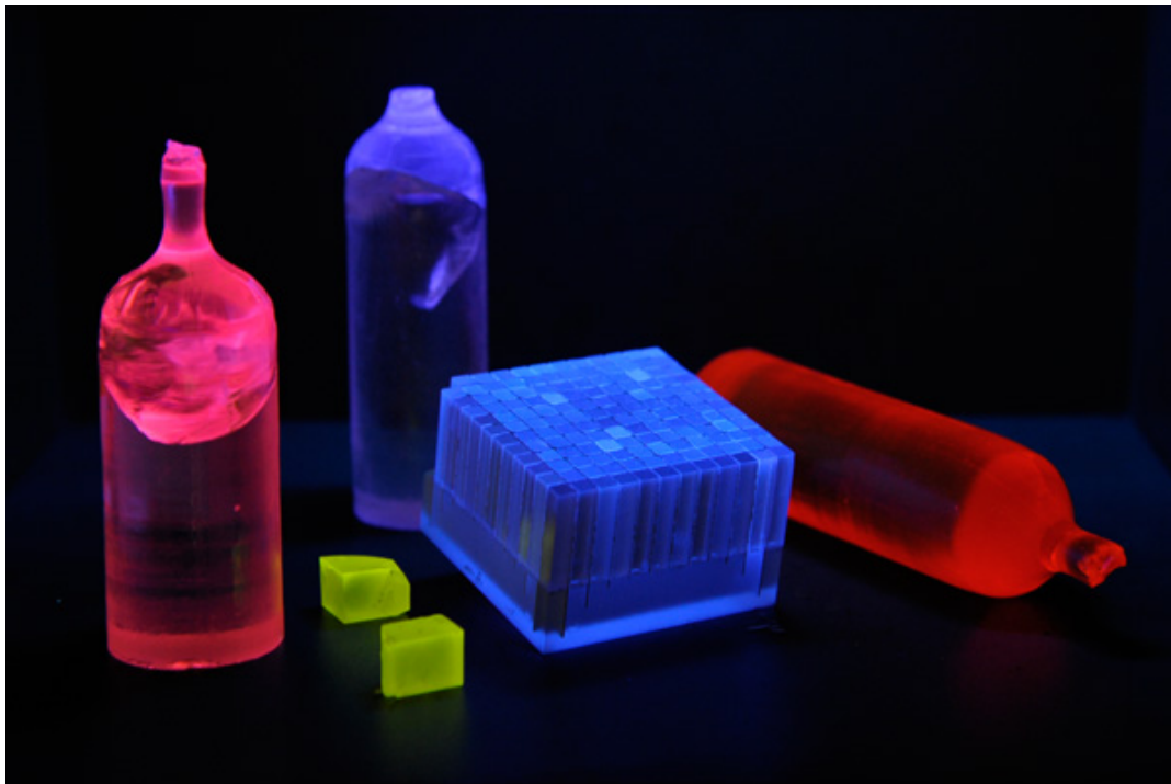
Figure 12: Scintillators illuminated with different wavelengths of color [52].
