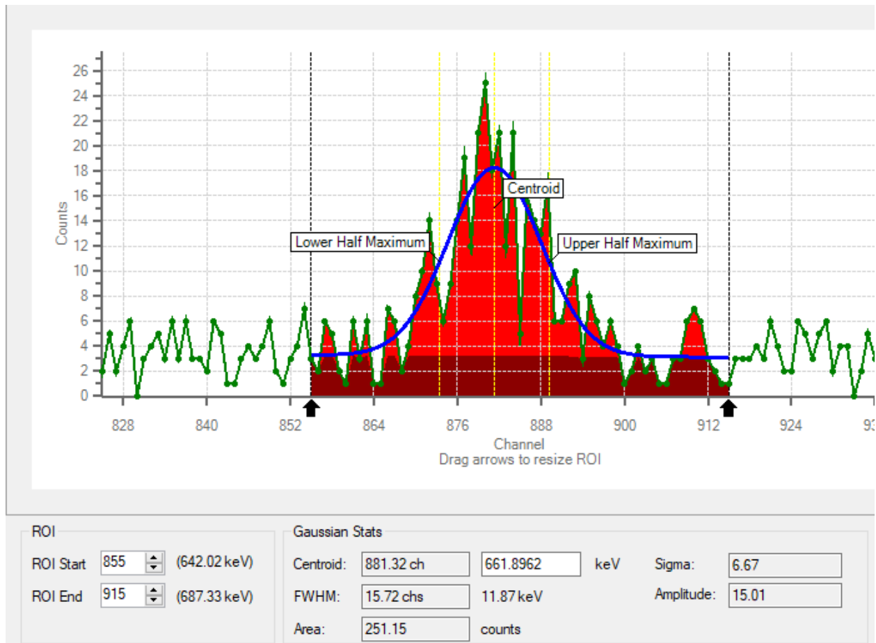
Figure 35: Gaussian stats of data from measurements with Zeolite attenuation from 12 inches.
