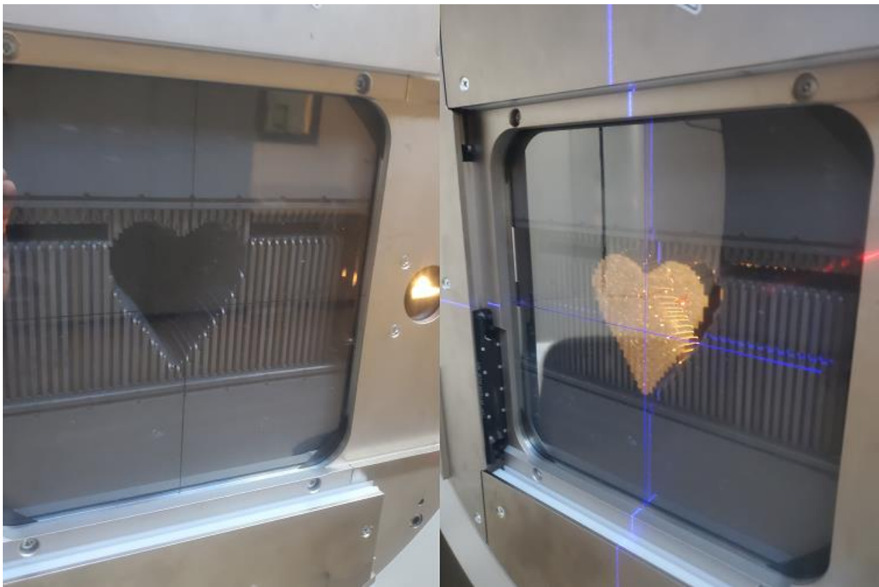
Figure 3. Example of multileaf collimator and its ability to shape output of radiation beams during treatment. MLCs are very versatile and can form very intricately, shown here by one forming a heart shape.
