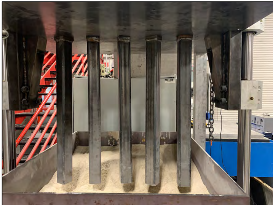
Figure 3-6: Tines Attached to Underside of the Tower Platform
