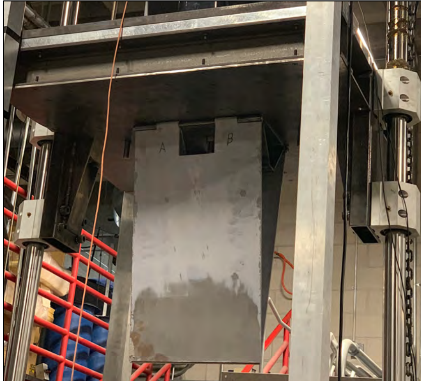
Figure 3-5: Wedge Attached to the Underside of the Tower Platform
