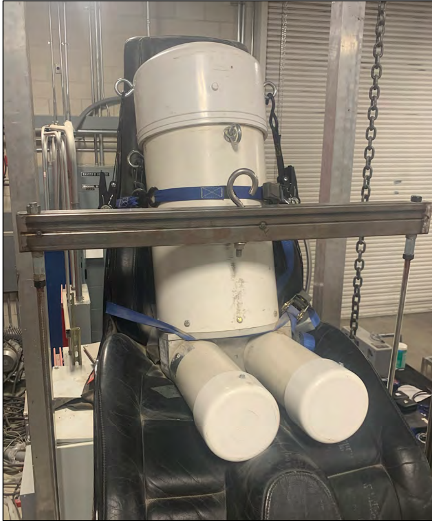
Figure 3-3: Test Payload Secured to the Test Seat
