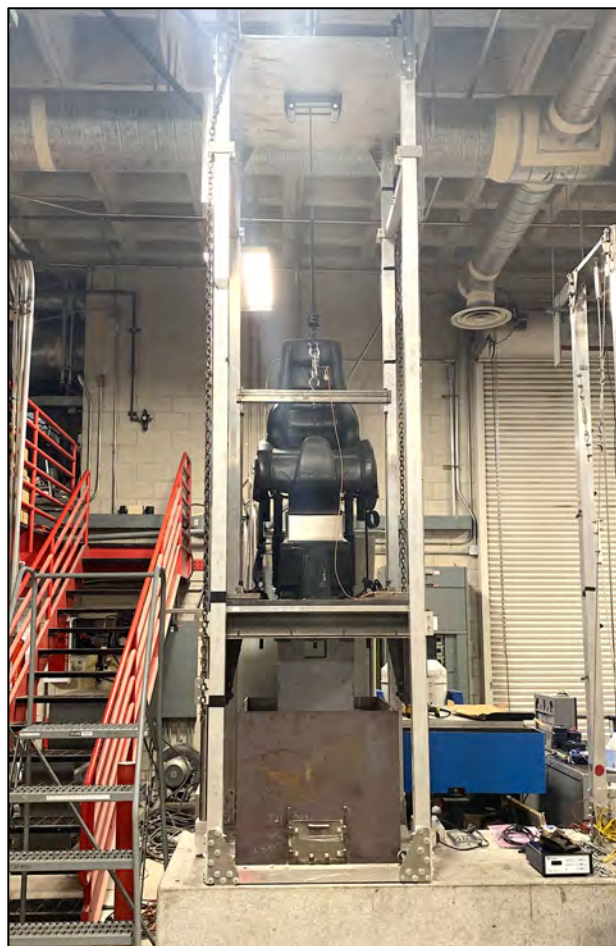
Figure 3-4: Drop Tower used for Single Impact Experimental Tests
