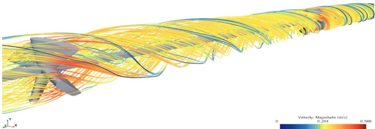
Figure 37 Streamline view showing swirls created by the vanes.
