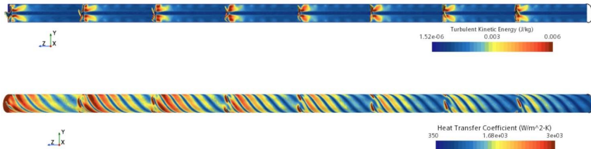
Figure 36 Scalar scene showing repeating pattern of increase in turbulent kinetic energy and heat transfer coefficient.
