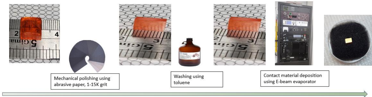
Figure 2.3. Schematic illustration of steps followed to fabricate MAPbBr 3 detectors.
