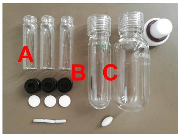
Scheme S1. Pictorial description of reaction tubes for the reaction. A is 2 dram vial, B is 15 mL flask, and C is 30 mL flask.
